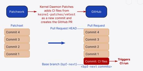
$\label{eq:file.github/workflows/test.yml from kernel-patches/vmtest tells GitHub to run the workflow on each PR creation/update$
